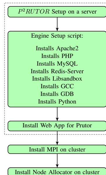
Fig. 5: Workflow of using P^2RUTOR for MPI Program Development and Execution on a Cluster.
