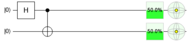
Fig. 5: The control qubit of a CNOT gate is placed in the superposition state: Bell state, simple example of entangled quantum states of two qubits
